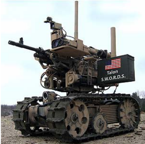
A SWORDS unit, equipped with the M249 Squad Automatic Weapon.
